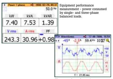
View waveforms for equipment checking and setup.
